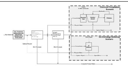
Figure 1. High-recovery process, including chemical precipitation and/or IX treatment.
